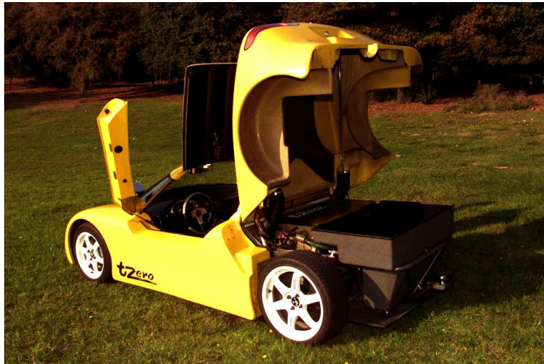
Figure 13. Doors, roof, and top opened. The trunk volume is 5.1 cu-ft – the same as that of a Mazda Miata
