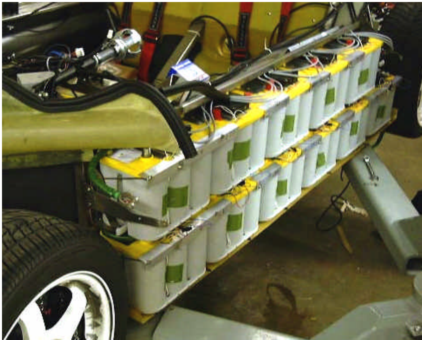
Figure 9. Battery packaging in side pods. The duct on the left is for battery pack cooling air.
