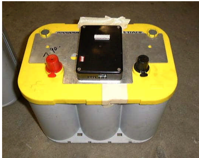
Figure 10. Optima 'yellow-top' battery with BatOpt unit mounted.
