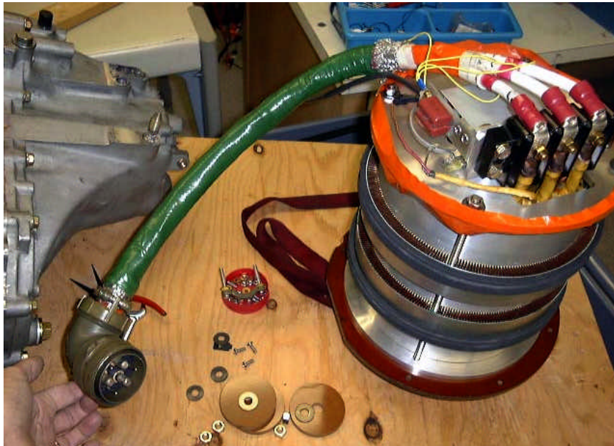
Figure 4. tzero's 177 kW (237 HP) induction motor.
