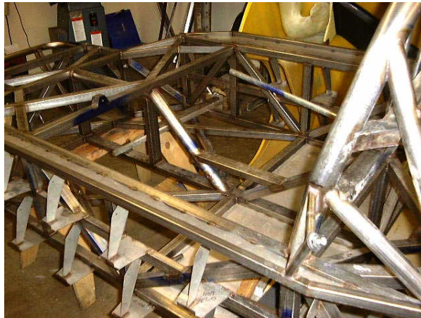
Figure 11. Frame looking forward from driver's side. Note battery hanger brackets
